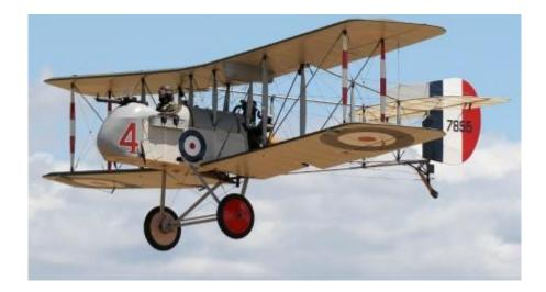
The DH.2 had sensitive controls and at a time when service training for pilots in the RFC was very poor it initially had a high accident rate, gaining the nickname "The Spinning Incinerator", but as familiarity with the type increased, it was recognised as very manoeuvrable and relatively easy to fly. The rear-mounted rotary engine made the DH.2 easy to stall, but also made it highly manoeuvrable.
